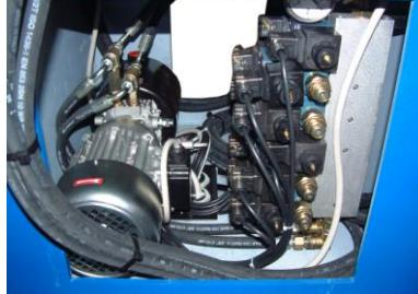
A photograph showing the internal components of a hydraulic unit. It includes various hoses, fittings, and mechanical parts housed within a metal frame. | <p>Centralina idraulica per espansione<br/>Hydraulic unit for expansion<br/>Hydraulische Aggregat für Spreizung<br/>Pompe hydraulique pour expansion</p> |
