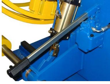
A close-up photograph showing a manual pump handle attached to a blue hydraulic component. A yellow hose is visible above the pump.                       | <p>Pompa manuale per espansione<br/>Manual pump for expansion<br/>Handpumpe für Spreizung<br/>Pompe manuelle pour expansion</p>                          |
