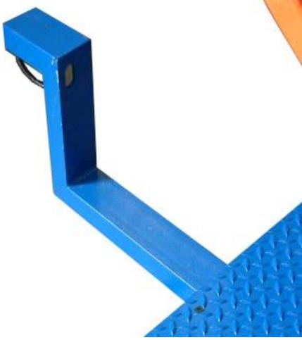
A photograph of a blue L-shaped metal bracket. A small black photocell assembly is mounted on one end of the vertical arm. The bracket is positioned against a white background. | <p>Fotocellula di stop rotazione aspo<br/>Photocell for decoiler rotation stop<br/>Photozelle für Haspeldrehung Halt<br/>Photocellule pour arrêter la rotation du dérouleur</p>        |
