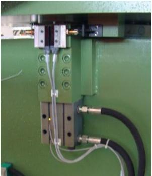
A photograph showing a green metal plate with various hydraulic components attached, including hoses and fittings.                                                                | <p>Blocco idraulico rotazione aspo<br/>Hydraulic system for decoiler rotation<br/>Hydraulisches System für die Haspeldrehung<br/>Système hydraulique pour la rotation du dérouleur</p> |
